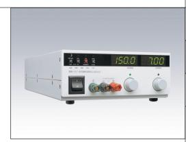
The XHR is power factor corrected for low current draw - only 11 amps at 120 volts AC for 1000 watts - and reduced generation of input current harmonics. Zero voltage or "soft switching" virtually eliminates switching transients for high efficiency, low noise and high reliability. It is also stackable, with a small footprint, front panel binding post connectors, and a low current requirement with universal input, making the XHR ideal for benchtop applications.
